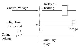
Wiring suggestion high temp limit when using electric heating.
